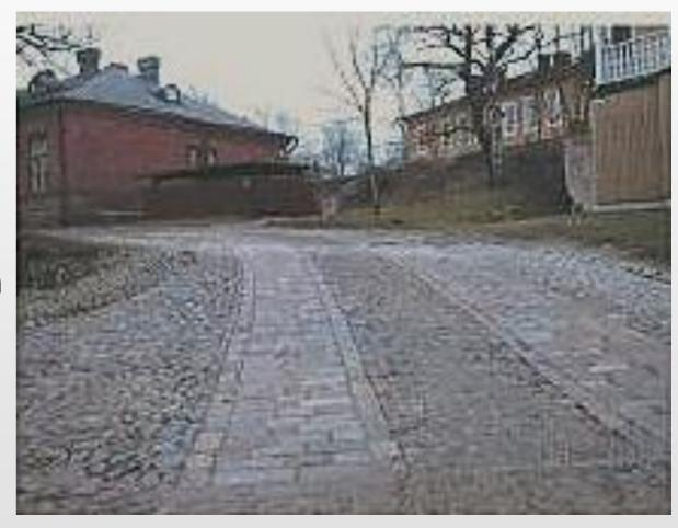
The cobblestone surface has been partially replaced by a more even flagstone surface to ease the accessibility on a wheel chair.
